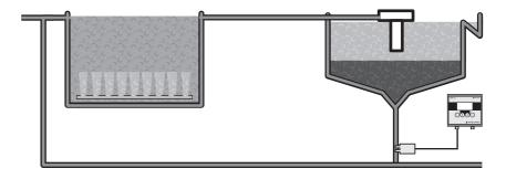
The TxPro-2 Transmitter, with a 4-Beam™ RD-262 Suspended Solids Sensor is used to monitor the settled sludge pumped out of the secondary clarifier. It transmits a current loop signal proportional to the solids concentration to remote control equipment. This data is used to determine sludge return rates, wasting rates and control of solids inventory.
