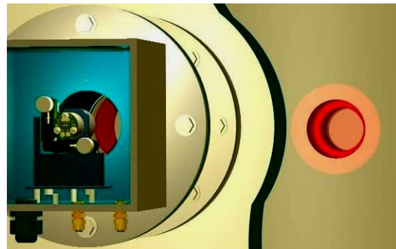
Figure 6.5 Centering Light Beam
