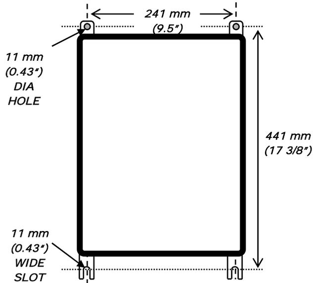
**Figure 12a. OFS Control Box Mounting Hole Pattern**
