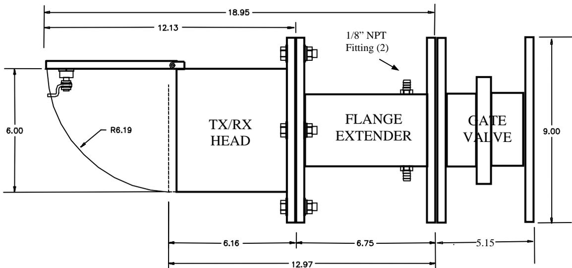
**Figure 11b: Top View Dimensions (inches) of OFS TX/RX Head with Extender**
