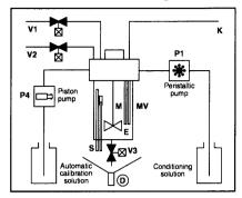
Rinsing valve : Automatic calibration Stirrer Siphon/overflow tube Sample valve gump
