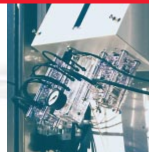
Tilt-out pump modules ease maintenance.
